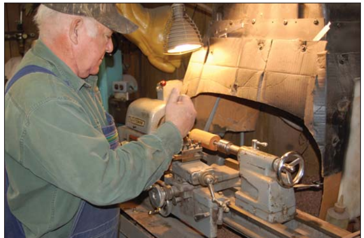
A tool-and-die maker, Norris is used to working in close tolerances. Below, Norris meticulously hand carves a call while a lathe is used to fashion the external shape of the call.
